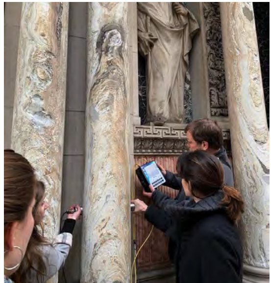
Ultrasound Pulse Velocity in use on the columns.
