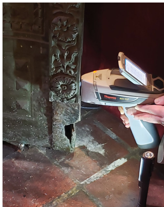
XRF Reading on Lost Decorative Door Trim.
